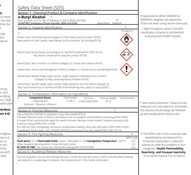
I How to clean up a spill. Always remove unprotected personnel from area and ensure all students are safe. Contain the spill with sand or absorbent materials.
