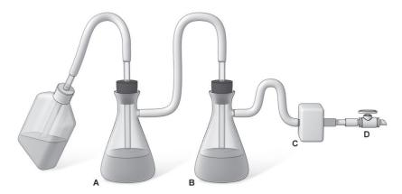
The disinfectant trap (B) should be an Erlenmeyer flask with a stopper having plastic tubing extending approximately halfway into the disinfectant solution. A 1-3 L Erlenmeyer flask filled approximately 1/10 - 1/4 full of disinfectant is recommended. Flasks should be plastic, plastic-coated glass or glass covered with safety netting or tape.
